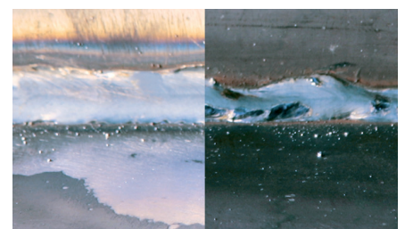
Surfaces descaled prior to welding result in clean welding seams (see image at left)
