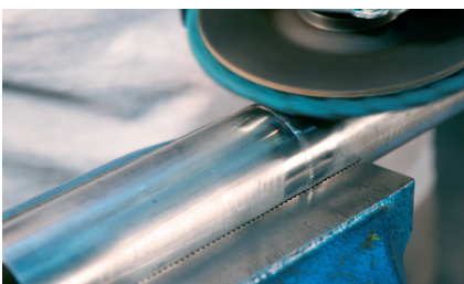
Sanding fine welding seams and removing thermal discoloration
